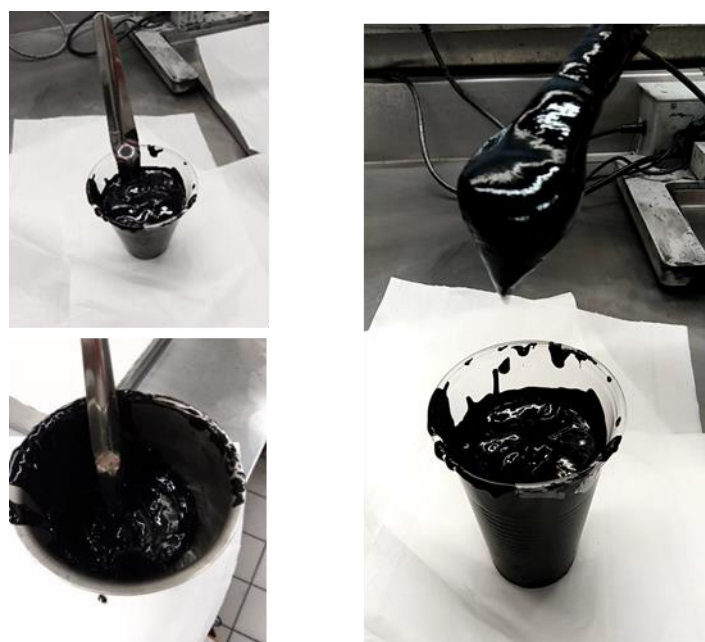
Figure 31: Lab scale preparation of electrode ink.
