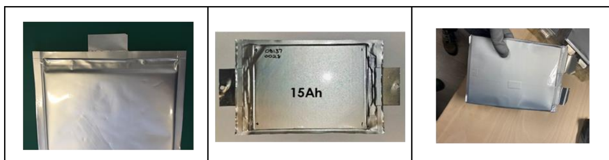
Figure 32: 3 generations of cells for DEMOBASE project with opposite (LS, LU and MU types) tabs and “rabbit type” tabs configuration (Mter type).
